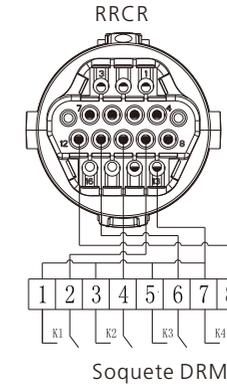
Fig6.20 Conexão inversor – RRCR
