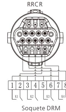
Fig. 6.16 Inversor – Conexão RRCR
